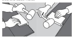
The elements of the last row are cut to size and inserted with a 10 mm gap to the wall
