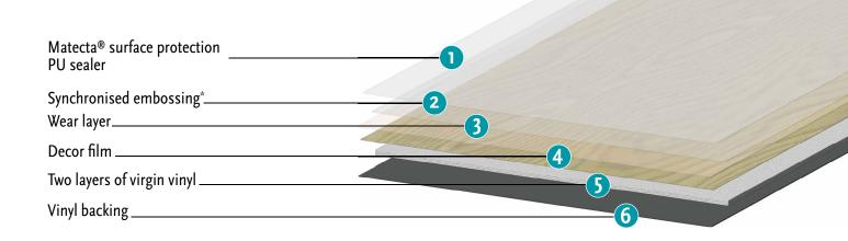
**Classic Vinyl** is a vinyl floor covering that is glued directly to the subfloor. It can also be used for rooms with hot water underfloor heating, among other things.
